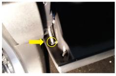
The cabin air filter housing is located behind the glovebox. To gain acces, the glovebox has to first be removed. Remove objects from compartment and unclip the strut shown in pic above.
