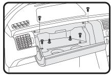
1: Open glove box and remove the 6 screws, glove box can then be removed.
