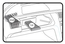
3: Pull the first used filter from the housing, slide the second filter to the right and pull out from housing
