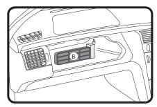
2: Lift the plastic filter cover mount (A), and pull filter cover (B) out.
