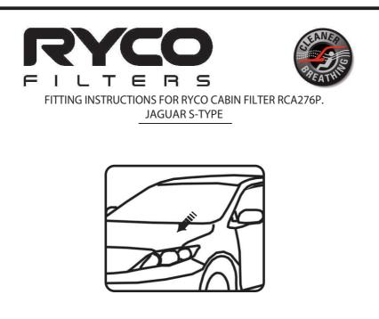
1. The cabin air filter is located in the engine bay below the cowl on the passenger side. The cowl requires to be removed.
