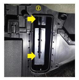
Once the cabin air filter housing lid is out of the way, the filter will be accesible. Pull the first filter out and then reach for the second one. Pay attention on how the filters sit in and replicate this with the new ones, making sure they are placed in the right air flow direction and lastly refit the housing lid.
