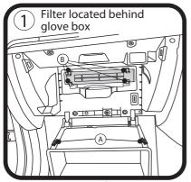
Undo 2 rubber lugs (A), pull glove box down, squeeze 2 handles (B) together & remove the filter cover.
