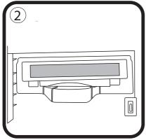
Pull used filter from housing, replace with Ryco RCA146P, Replace previously removed parts.
