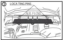
FIT THE NEW FILTER BY LOCATING THE TWO PINS ON THE BOTTOM SIDE OF THE FILTER FRAME INTO THE HOUSING, CLIP THE TOP EDGE IN PLACE AND REFIT THE COVER.
