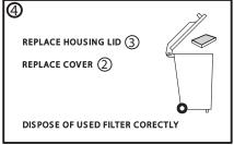
PULL USED FILTER FROM HOUSING AND REPLACE WITH NEW FILTER, NOTE DIRECTION OF AIR FLOW..
