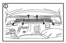
USING SUITABLE ALLEN KEY UNDO THE 6 SCREWS AND REMOVE THE COVER.
