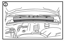
LIFT COVER TO OPEN HOUSING AND REMOVE USED FILTER BY UNCLIPPING FROM THE TOP EDGE AND PIVOT FORWARD TO REMOVE FROM HOUSING.
