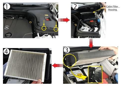
1. Locate the cabin filter housing cover at the passenger side under the bonnet. Remove the two clips (Fig 1.) then open the cover.
