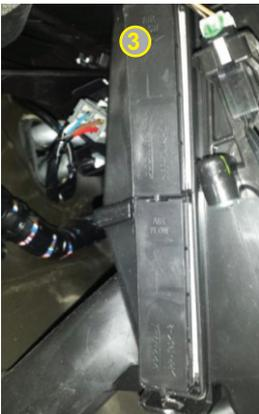
Filter comes in two pieces. Slide out the bottom one and then the top one.
