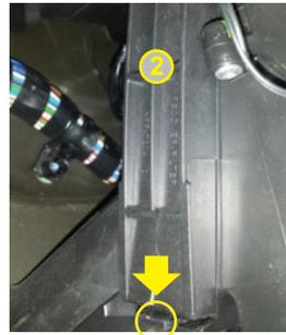
Move protective foam out of the way and proceed to release the cabin air filter housing lid by pressing clip as indicated on the picture.
