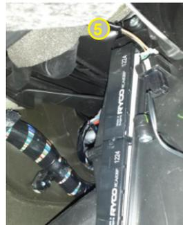
Slide the top Ryco Filter first and push it upwards. If placed properly it should stay up by itself, then slide bottom one. Push in gently both filters until it clicks in. The housing lid will then easily fit back. The lid won't secure until filters are in the right position.
