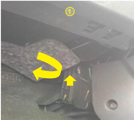
The cabin air filter is located in the footwell area against the centre console as indicated in the pic.
