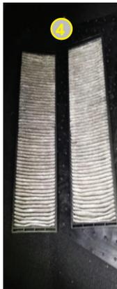
Note how the old filter was fitted and pay attention to air flow direction and organize the Ryco Filters the same way.
