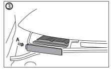
PUSH IN AT ARROW "A" AND PULL HOUSING LID OUT TOWARDS FRONT OF VEHICLE.
