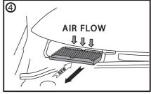
PULL USED FILTER FROM HOUSING AND REPLACE WITH NEW FILTER, NOTE DIRECTION OF AIR FLOW...
