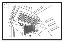
Push new Ryco RCA112P filter into housing.
