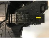
2. Slide the cabin filter cover to the rear of the vehicle. Remove the cover and filter.
