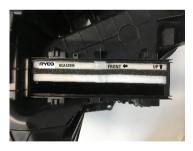
4.Insert the new filter into the housing. Look for UP and FRONT arrows to identify position direction. Refit all components in reverse order.
