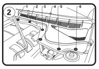
2: Remove the 6 scrivets, using a flat bladed screwdriver, insert blade into slot and twist to lift centre piece, then remove scrivet
