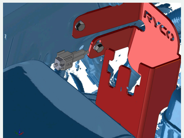
FIGURE 2C CATCH CAN BRACKET SLOT B & C INSTALLED
