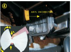
Release the housing cover by depressing the locking tab at the lower end and sliding it downwards. Carefully tuck out the bottom corner of old filter and squeeze & pull it out.
