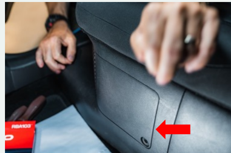
STEP 4A Using flat head screw driver or hands, wedge in-between around perimeter of battery filter OEM housing flap and back seat to begin removal of housing flap - then gently pull open flap to release remaining tabs.
