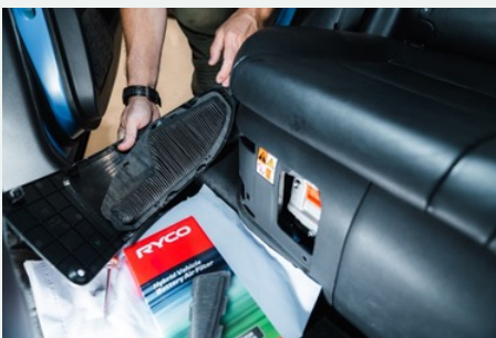
STEP 5B Once flap is released, remove old battery filter by releasing the filter from the tabs holding it in place by pulling away from OEM housing flap. Then install new battery air filter in same orientation as old filter was installed.
