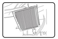
2: Lift front of cover to remove, turn cover over to remove filter.
