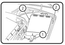
1: Open engine hood to vertical position. Unscrew plastic nut (1). Release both snap fastners (2) on filter housing.
