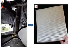
Slide the filter out carefully to avoid accumulated debris from being spread around. Disconnect the connector at the back of the housing if if the cable is difficult to lift and slide the filter underneath. Insert the new cabin air filter making sure it is in the right air flow direction (See side of filter) and refit all components in reverse order.
