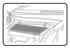
2: Remove used filter, fit new ryco filter.
