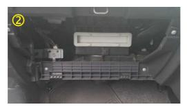
Pull out to remove the old cabin filter Then fit new filter into the housing Male sure the filter flow mark is facing up.
