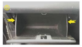
The cabin air filter is located behind the glove compartment. Push each side of glove compartment to release, then remove glove compartment.
