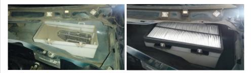
Some vehicles will not have had a cabin air filter installed new from the factory, however the housing is there to accomodate a cabin air filter. Make sure the housing is cleaned properly and insert the new Ryco cabin air filter. To fit, slide the filter in making sure the locating tabs at the rear of the filter frame locate inside the rear tabs of the housing and press the filter down until it clicks in the two front tabs.
