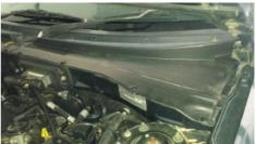
Remove the 4 plastic clips holding the bottom of the plastic trim. Now pull the trim out. The cabin filter housing lid will be visible at this point, it is secured by two plastic clips. Remove clips and pull out the lid.
