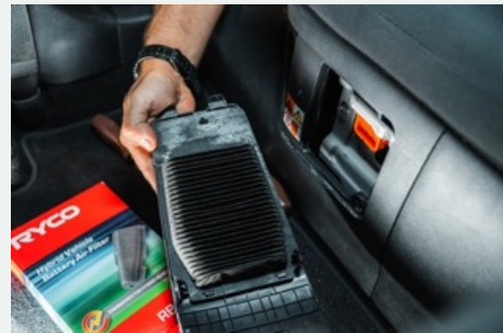
STEP 5A Once flap is released, remove old battery filter by releasing the filter from the tabs holding it in place by pulling away from OEM housing flap. Then install new battery air filter in same orientation as old filter was installed.
