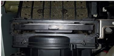
5. Grab the cabin air filter tray and slide it out slowly to avoid any loose debris from spreading around.
