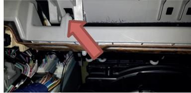
2. Before opening the compartment lid, the retaining lugs holding it in position need to be removed. With a flat screw driver lever the lug from its head out of the slot. Do the same with the other side. Once both are out, open the lid and slowly remove it.
