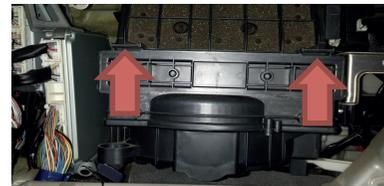
4. Once the compartment is removed, the cabin air filter housing is easily visible sitting on top of the blower fan. Unclip the lid from the location indicated in the picture above.
