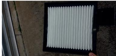
6. Clean the housing and the tray and then slide the new filter through the tray channel making sure the filter is facing in the right air flow direction. Refit all components in reverse order.
