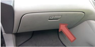
1. The cabin air filter is located behind the glove box compartment. Follow the instruction to replace the element.
