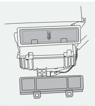
**STEP 3**Unclip filter cover and remove, pull used filter out of housing and replace with new Ryco filter.
