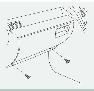
**STEP 1**Undo the two screws at bottom of glove box as shown.
