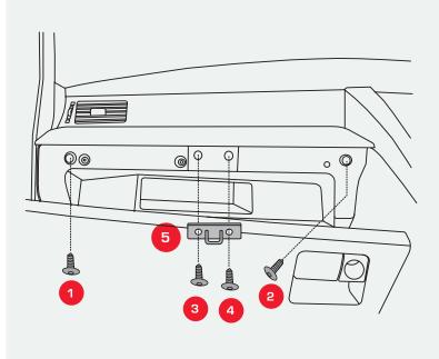
Open glove box, and undo the four screws at top of glove box as shown, screws 3 & 4 retain staple (5) for glove box lock, lower glove box to access filter housing, disconnect glove box light from back of glove box.
