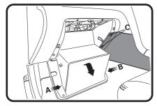
1: Open glove box, push each side of glove box (A & B) to release catches, glove box can then be rolled down to 180° position. Unclip trim panel (push / pull clips) (C) to reveal hidden screw.
